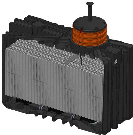
The ClearFox® fixed-bed modules are fully equipped bioreactors in a high-quality PE mold. All equipment parts, such as aerator plates, distribution systems and the fixed bed material in a cubic tank are part of the pre-installed standard equipment of the high-performance bioreactors. The typical application is the reduction of carbon and/or nitrogen concentration from any type of pre-treated (solids removed) wastewater of industrial or municipal nature.
