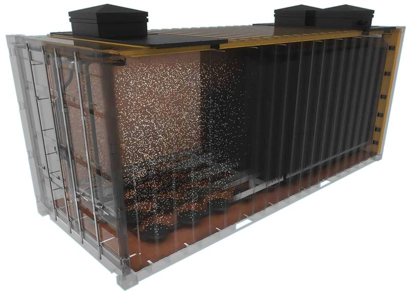
The ClearFox® fixed-bed modules are fully equipped bioreactors in a high-quality PE tank. All equipment parts, such as aerator plates, distribution systems and the fixed-bed material in a cubic tank are part of the pre-installed standard equipment of the high-performance bioreactors.
