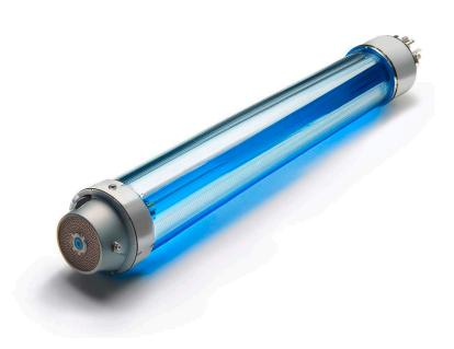
ClearFox® UV treatment modules are characterized by an extraordinarily high disinfection performance with a compact design and low energy consumption. They are designed in accordance with applicable laws, standards and guidelines. They consist of a stainless steel pipe reactor where the pretreated wastewater passes an highly efficient UV lamp. The water flows by gravity or can be pumped. The reactor is included. Downstream after Clearfox DAF, FBR and SBR.
