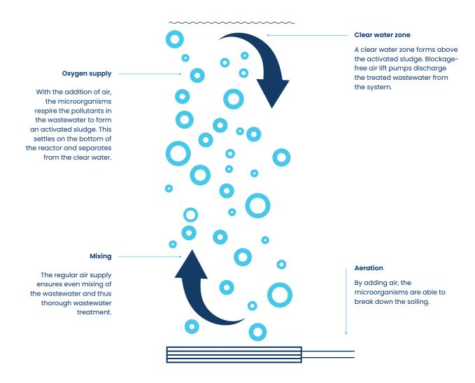
ClearFox® SBR is a proven process for **biological wastewater treatment**. By regularly aerating the wastewater, microorganisms are able to break down the pollutants in the wastewater. These form an **activated sludge** that settles to the bottom of the tank and thus separates from the treated wastewater. An **intelligent control system** adapts the cleaning cycle to fluctuating wastewater inflows and dirt loads. It thus achieves any prescribed degree of purification.
