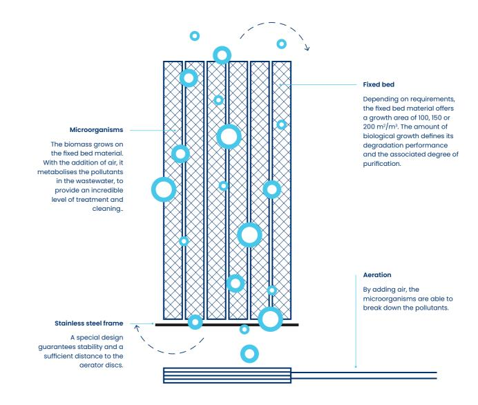
The ClearFox® FBBR is the most efficient and robust process for biological wastewater treatment on the international market. It is a modification of the well-known fixed-bed process used worldwide. By utilising special cascades and aeration sequences, the ClearFox® fixed bed biological reactor treats municipal and industrial wastewater. This method is far more stable than typical activated sludge processes and produces less sludge than conventional biological wastewater treatment methods.
