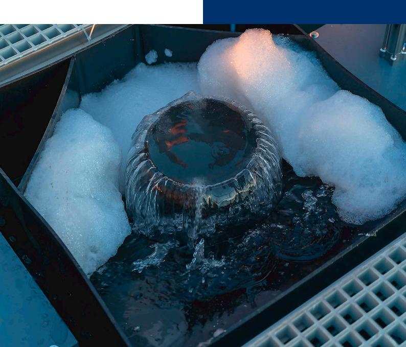
ClearFox® DAF dissolved air flotation is a physical-chemical process for the separation of a wide range of pollutants from wastewater. The specially developed flotation reactor enables efficient separation of pollutants from wastewater, with lower OPEX costs than a standard dissolved air flotation system.
