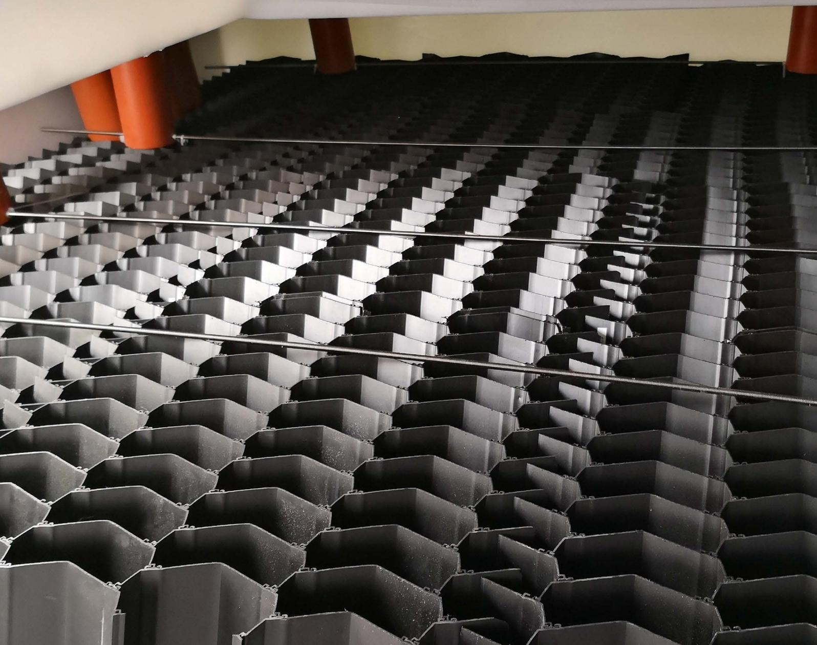
ClearFox® Clarifier is a separation process for removing particles from liquids. A clarifier is mainly used after biological treatment to clarify final effluent.
