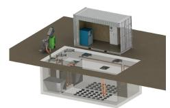
QuickOne SBR SBR proccess in single chamber tank with sludge stabilisation.
