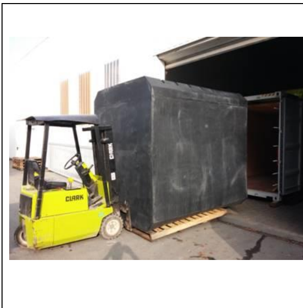
biomodule installation into a seacontainer
