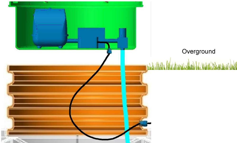
7. Screw down the inserted control module with the 6 screws , please make sure that is in the right position and also the fixing angles !
