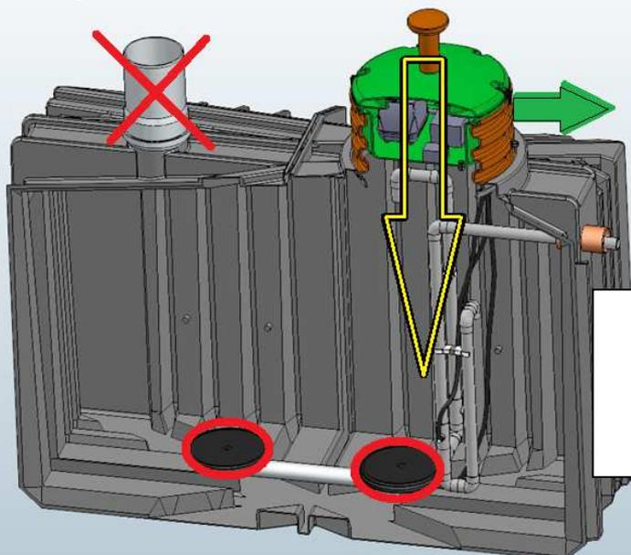
**Be carefully with all installed equipment, especially with the aeration discs on the tank ground. It could be damaged through wrong handling of the suction lance!**
