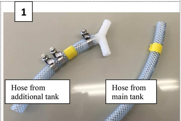
2. Remove the three stainless steel hose clamps and the plastic distributor from the hose. →Picture 2
