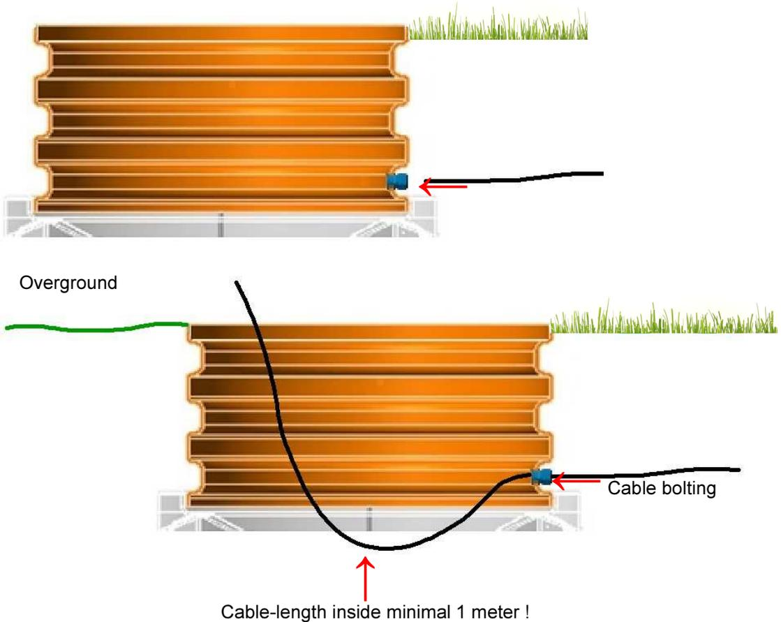
5. Implement the cable into the control module, and connect it with the power socket. At next, tie up the cable-bolting (see sketch overhead), for saving the control module against wetness.
