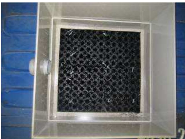
top view into fixed bed reactor , risers in PP 600 mm, foam tube
