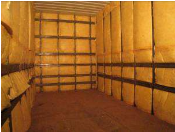
side insulation in fixed bed container with 120 mm glasswool between the reinforcement
