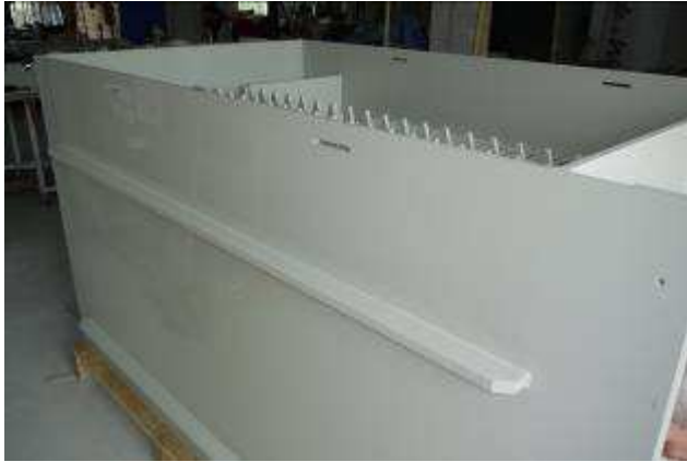
lamella module 8 m 3 /hour, 1.200 people equivalent , before installation into 20 feet container
