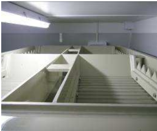
lamella clarifier top view inside container full insulation 20 ft
